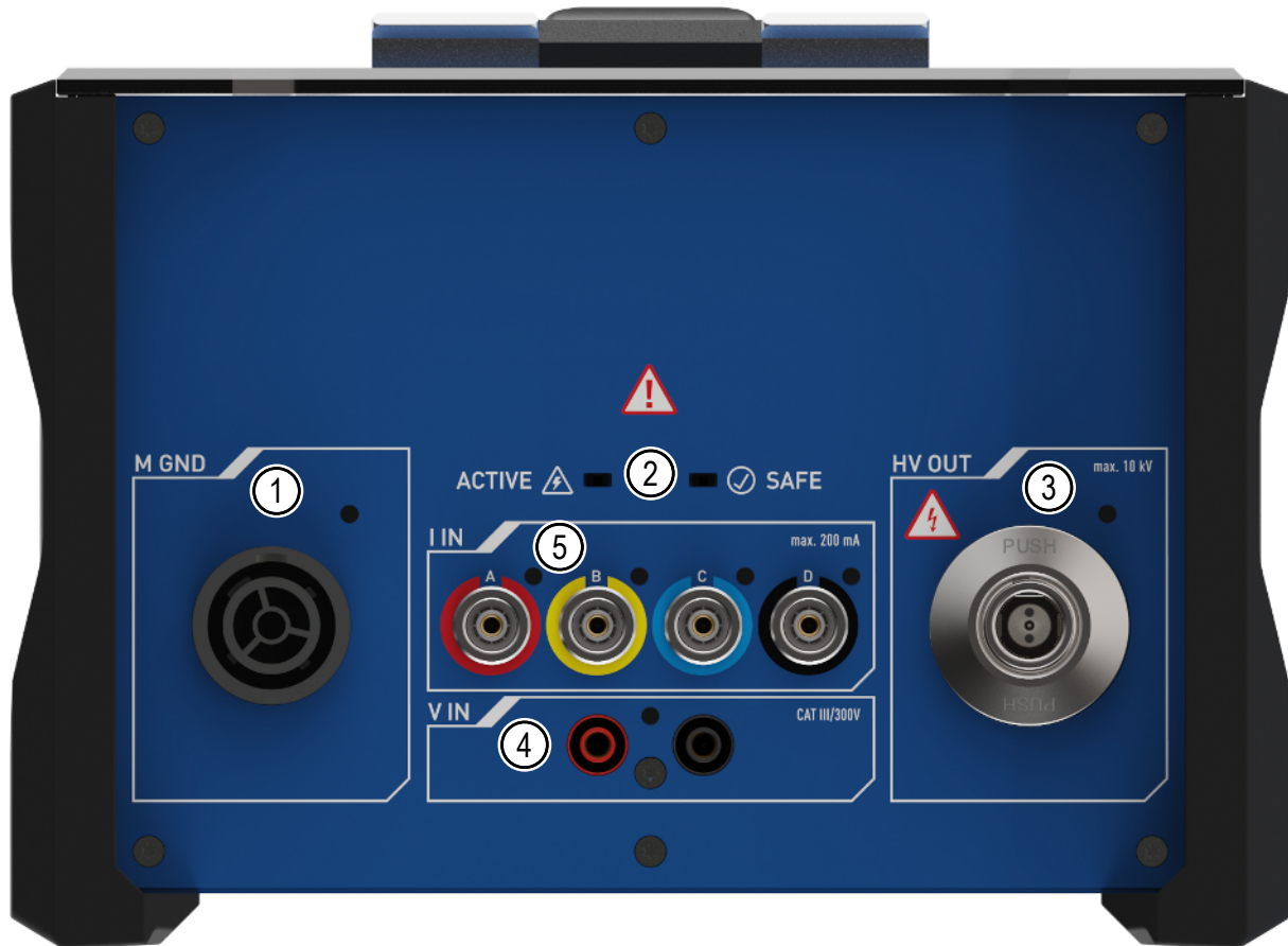
Figure 4-2: HVX10 left side panel with grounding terminal, measurement inputs and high-voltage output
