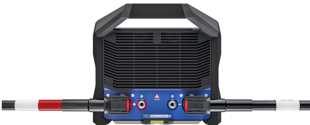
Figure 3-6: 1 000 A AC/DC High Current Module cables in locked state
